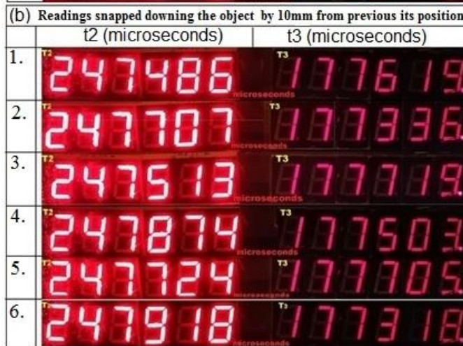
Fig. 8. Photos of displays of readings of microsecond timers (a) for first position, (b) for second position after downing the free fall object by 10mm
