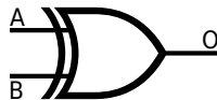
Figure 3: 2-input XOR gate; A and B supply the inputs, and O receives the output.
